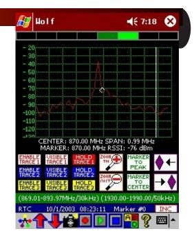
Use the "marker to peak" button to move the diamond marker to the current highest dBm valued point. Use the "marker to center" button to move the diamond marker to the center of the currently displayed section.
